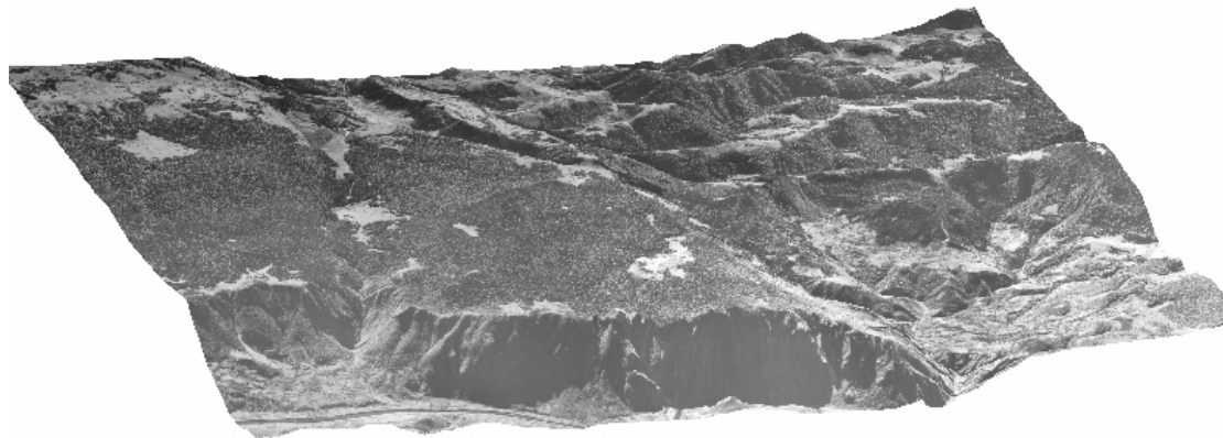
Fig. 7. Aerial photo (of part of Tara NP) georeferenced and joined to DEM (N view)
