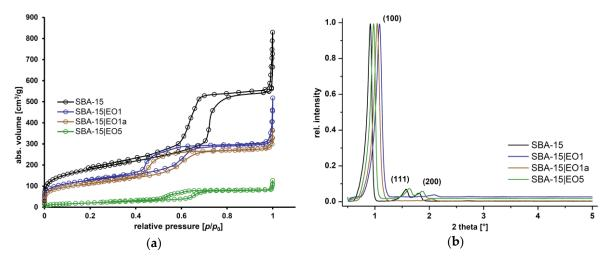
**Figure 2.** N<sub>2</sub> adsorption-desorption isotherms (**a**) and small-angle X-ray scattering (SAXS) patterns (**b**) of SBA-15 and SBA-15 | EOn (n = 1, 1a and 5).
