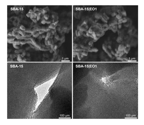
Figure 1. SEM (upper) and TEM images (lower) of SBA-15 and SBA-15 | EO1, as example.
