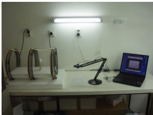
Figure 1. ELF-MF apparatus (left), camera (middle) above Petri dishes, and computer (right) for locomotor activity recording.
