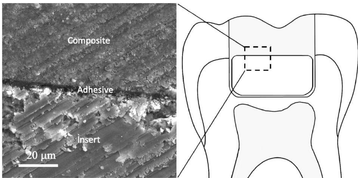
Figure 1. Schematic representation of cross-section of a molar restored by the newly proposed protocol involving hydroxyapatite-based dental insert, and FE-SEM micrograph of the composite-adhesive-insert interface. The dental insert based on hydroxyapatite doped with magnesium is bonded with Filtek Z_250 dental composite by Single Bond Universal adhesive applied by total-etch protocol.
