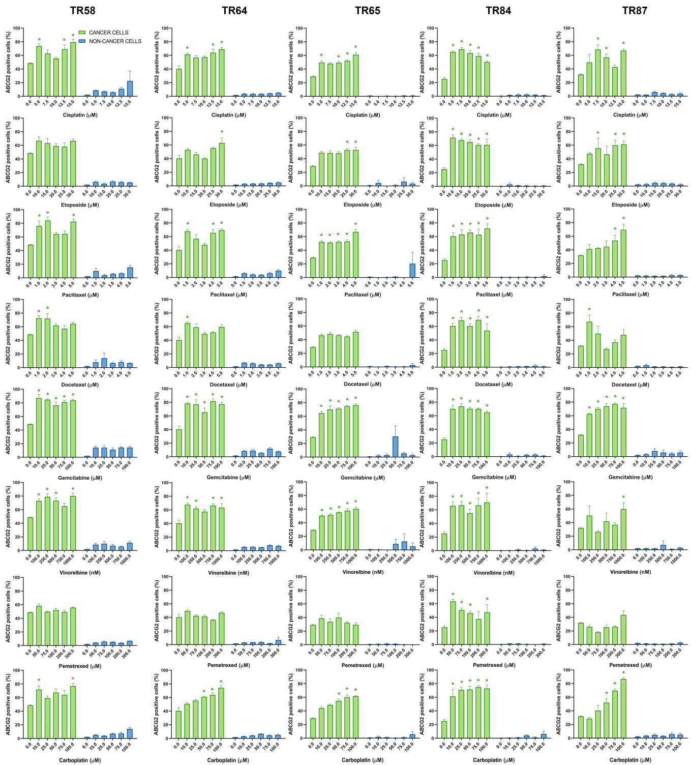
Figure 7. Patient-derived NSCLC cultures expressing ABCG2 after treatment with chemotherapeutics. CK8/18 antibody was used to distinguish cancer cells from non-cancer cells in mixed culture. Graphs show the percentage of ABCG2-positive cells for each experimental condition. Data are presented as mean ± SEM ( n = 4 ). A statistically significant difference between control and treated groups that showed an increase in ABCG2 expression of at least 20% is indicated as * ( p < 0.05 ).
